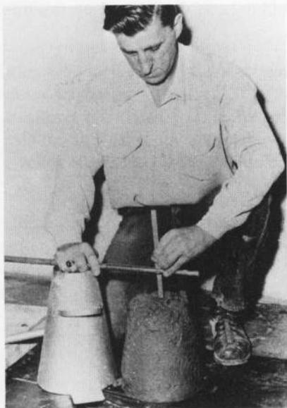
Measuring the slump after subsidence
