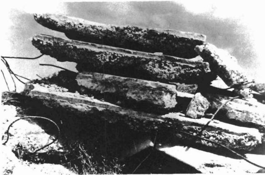
Figure 137.—A chute lining that failed because of almost complete lack of consolidation except at the surface. Most of the reinforcement steel was found to be in a useless location at the bottom of the slab. PX-D-20776.
