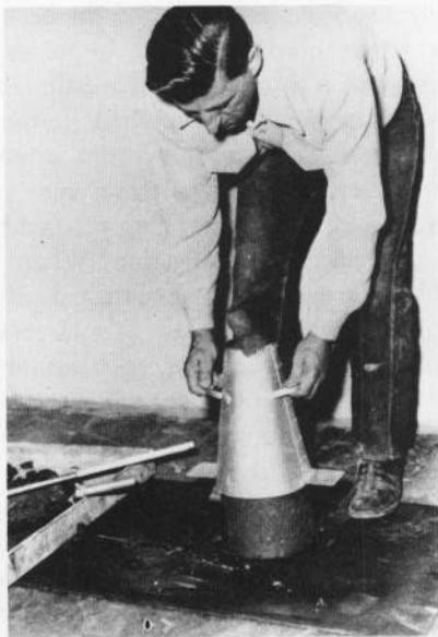
Slow, steady, vertical removal of the mold
